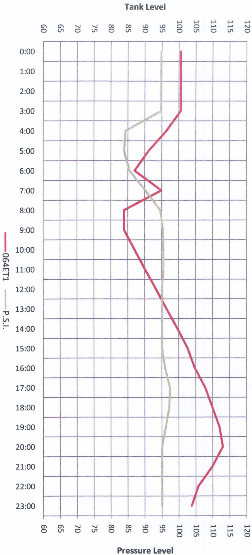
Facility 064 Elevated Tank & Pressure Levels August 21, 2009
